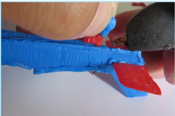
Attach the triangle piece to the bottom of the plane just ahead of the rear wings.
