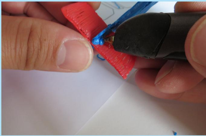
Slide the back wing in the slot under the tail of the plane and doodle it into place.
