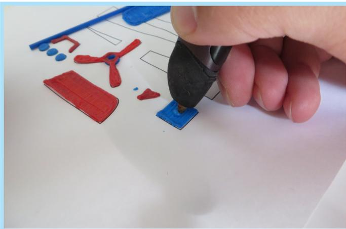
Cut a small piece of fresh plastic, then extrude a ball of plastic in the center of the square piece.
