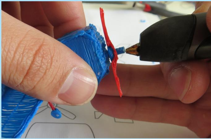
Slide the propeller onto the front of the plane and extrude some plastic on it to lock it in.
