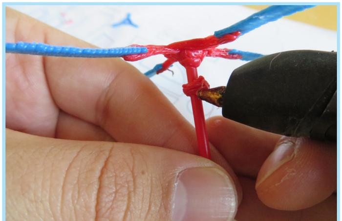
Doodle a ring around the strand about 1/2 cm from the propellers. Hold the pen in place while twisting.
